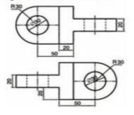
Draw the Isometric view object shown in of the following orthographic views and show the dimensions.
